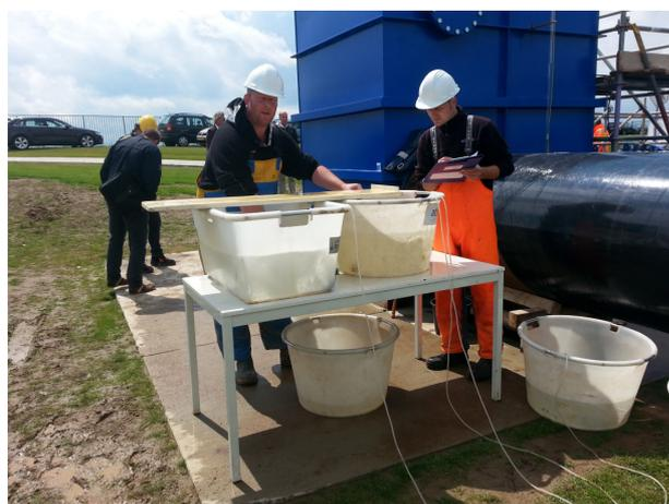
Examining fish for damage following testing carried out at the Pro-Tide NL site at the Maurik hydropower plant.
